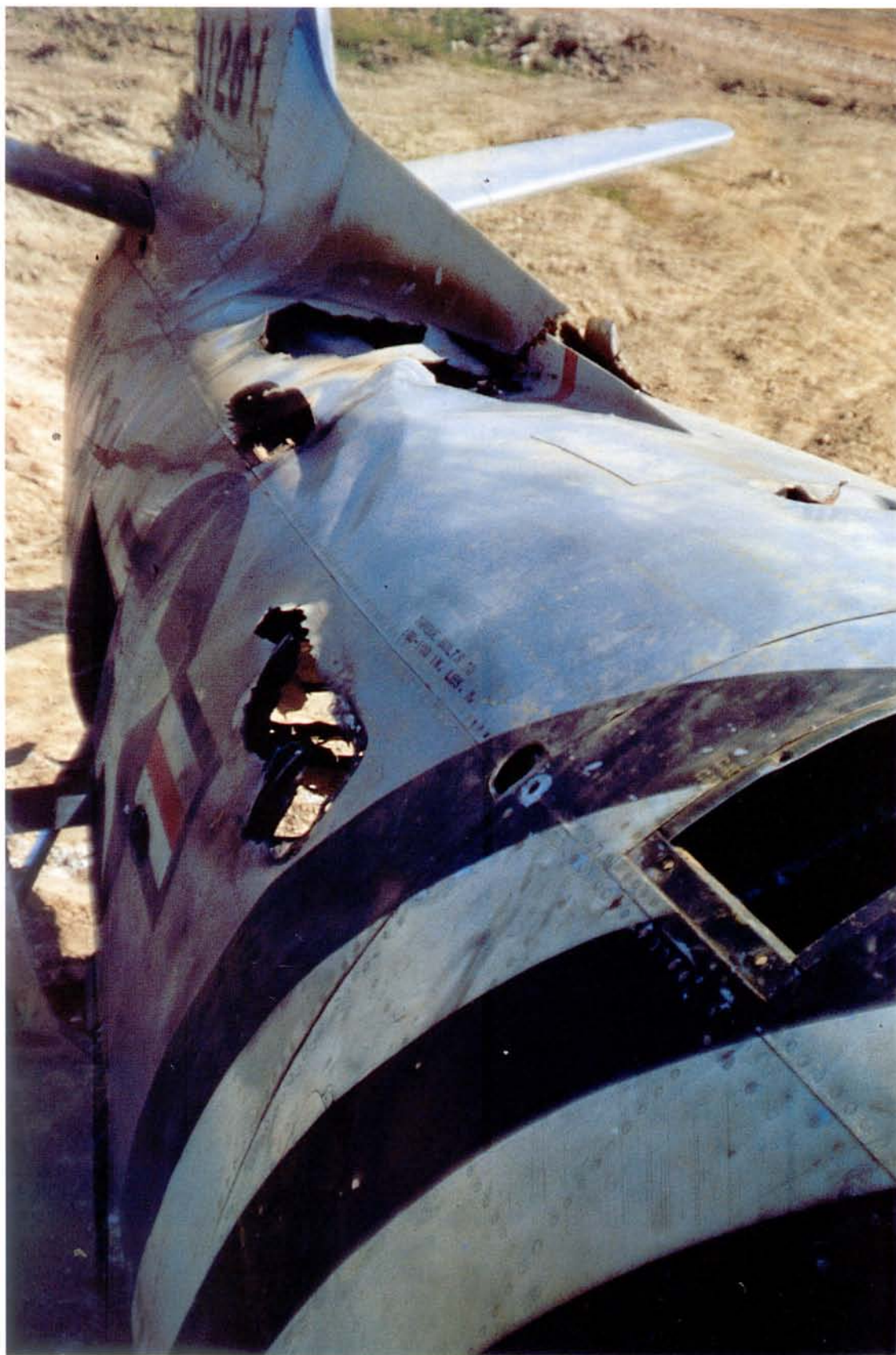
LEFT Lt Col Glenn Eagleston was an eyewitness to the MiG-15's devastating firepower six months into the 4th FIW's tour in Korea. It did not take too many hits from the slow-firing 37 mm N-37 cannon to inflict heavy damage, or even to blow a Sabre's wing off. Eagleston flew his F-86 safely back to Johnson AB, Japan, where it was declared fit only for the salvaging of spare parts (John Henderson)
