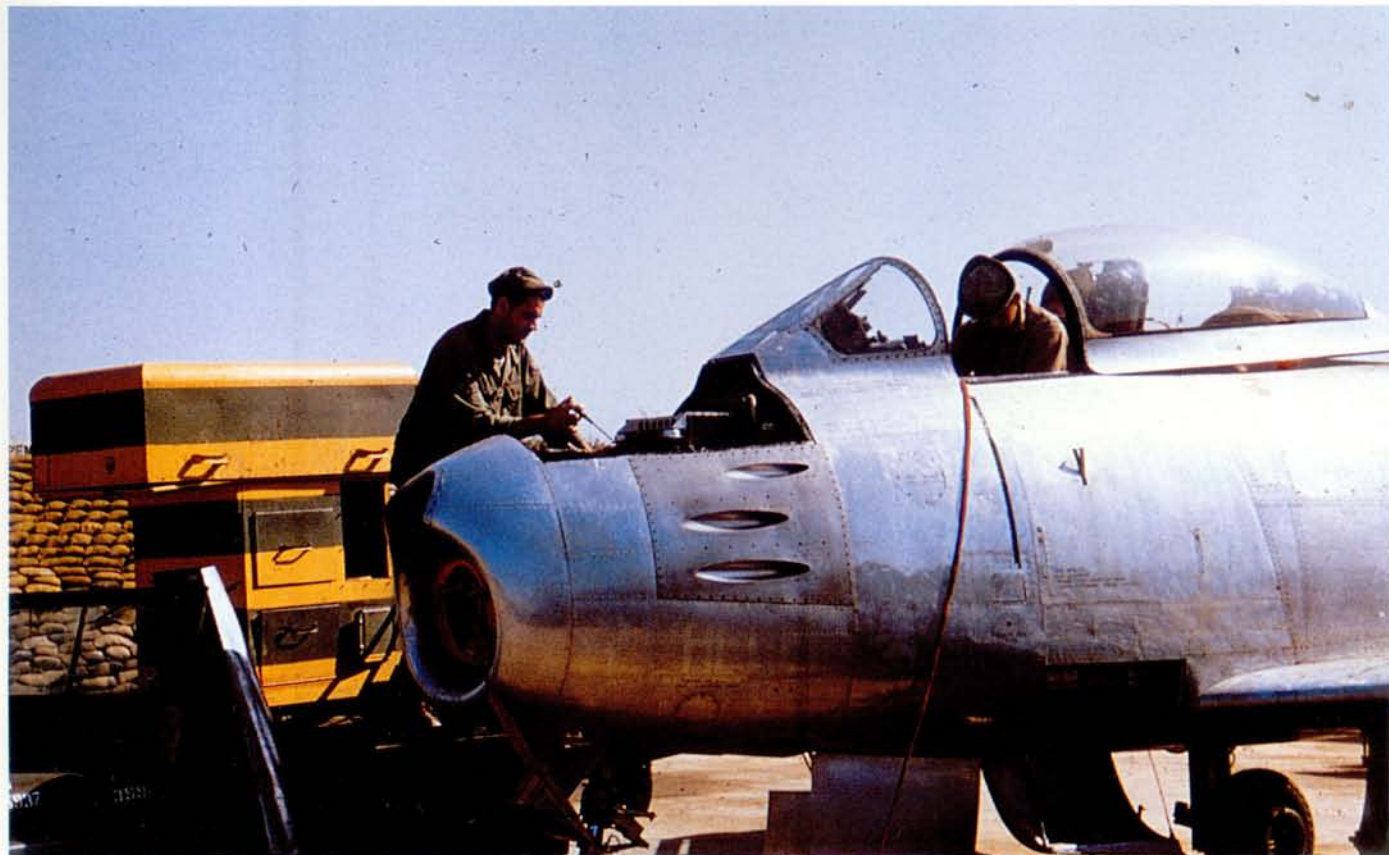
ABOVE In the summer of 1953 the large number of MiG-15s available to the enemy placed a heavy maintenance burden on the 4th FIG, because its Sabres had to be ready to fly combat air patrols day after day. There were many more pilots than aircraft to crew them, and they were anxious to fly the missions, complete their tour and go home. These men are servicing the aircraft's radio transmitter unit, having first removed the electronics bay access panel (Bert Beecroft)
