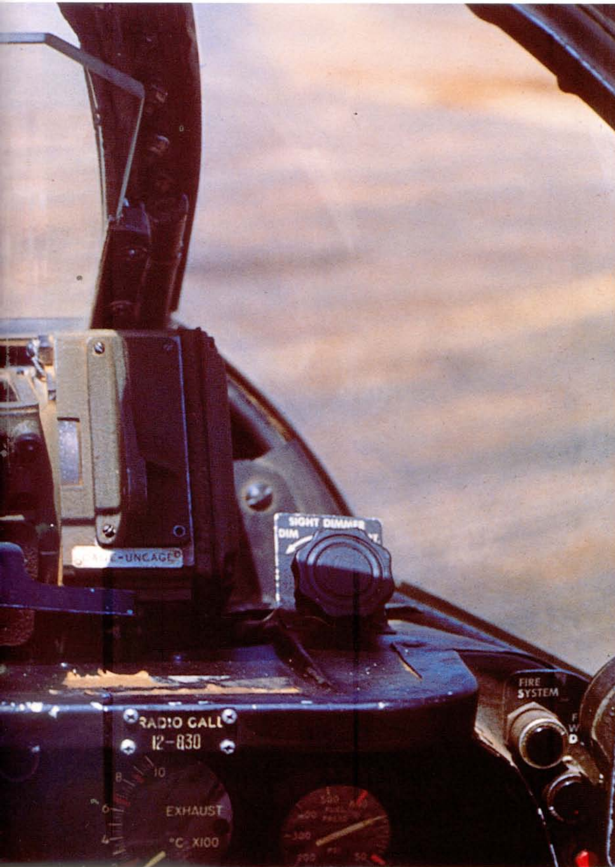
The pilot's view of the A-1CM gunsight mounted in a 4th FIG F-86E. The first 530 A-models off the assembly line had the Mark 18 sight fitted, with the more complex A-1CM only being installed in the final 24 F-86As built, and on all F-86Es. Although the Sabre had radar for automatic ranging, its complexity made maintenance difficult in the field (Ernie Atkinson)
