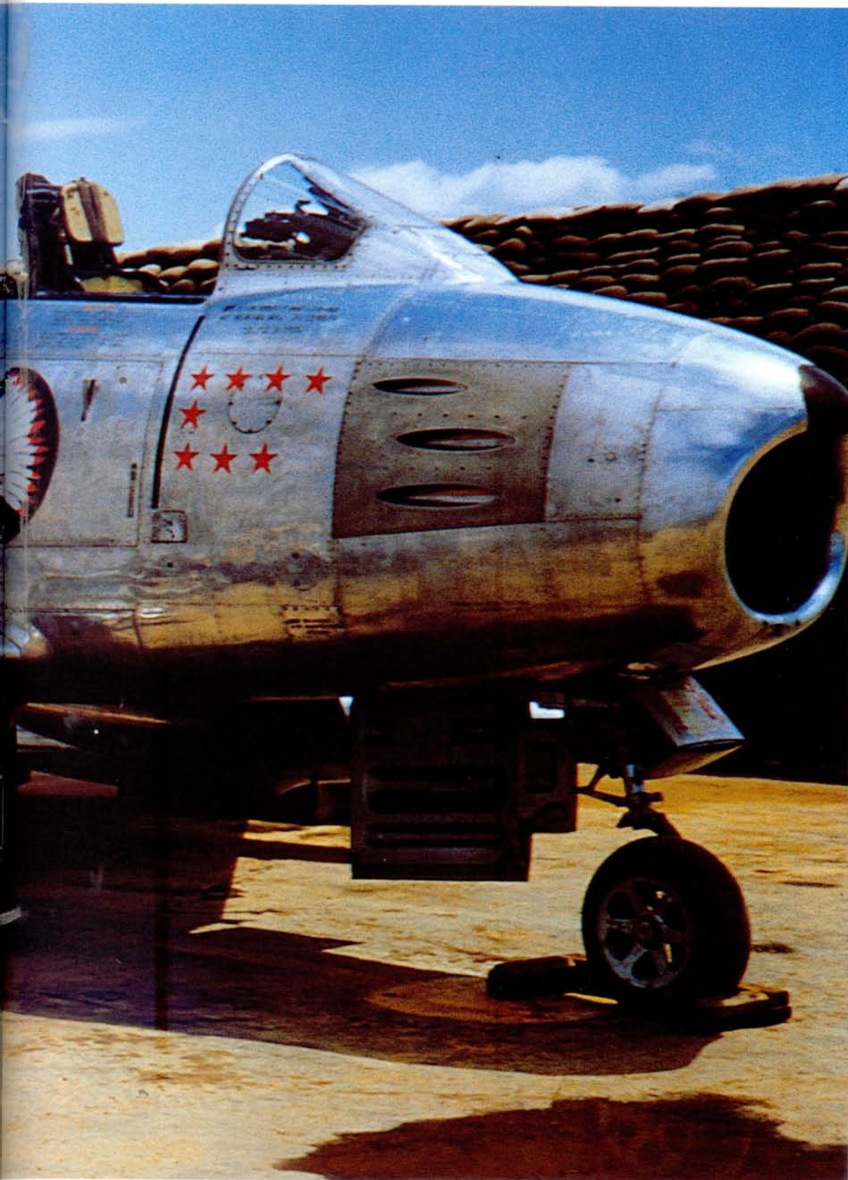
335th FIS groundcrew remove the canopy from Maj Jack Mass's Sabre. Four of the kill symbols painted on the fuselage were credited to him. Some of the highest scoring F-86s were flown by several different pilots. This particular F-86F-10 served with the 51st FIW after the war, before being given to the Nationalist Chinese (Norman Green)
