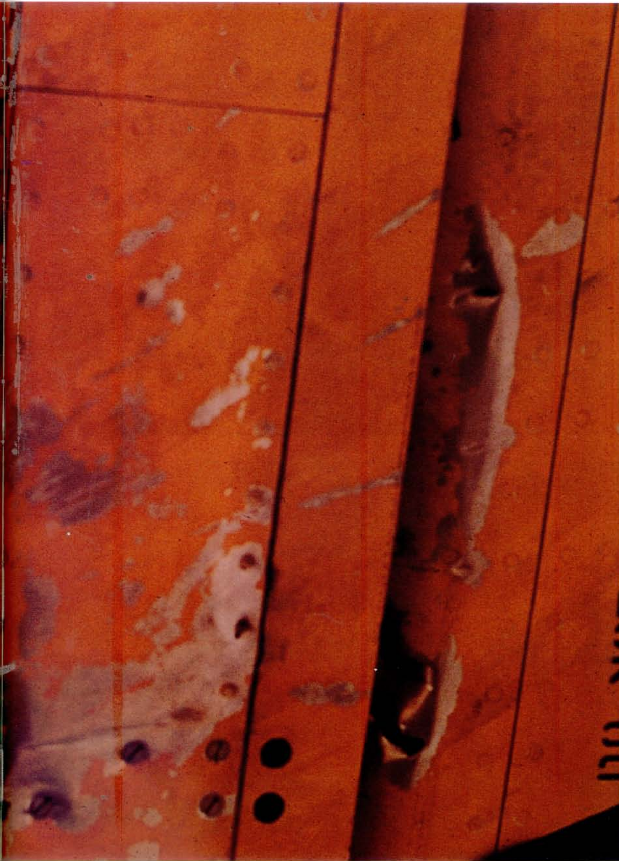
Combat-seasoned 335th FIS pilot Lt Martin Bambrick examines the large hole made by a 37 mm shell fired from an NR-37 cannon fitted in the nose of a MiG-15 in June 1952. It only took a round or two from this heavy calibre weapon to blow an F-86 out of the sky. Indeed, Maj Felix Asla, 336th FIS CO, was killed when a shell ripped a wing off of his Sabre on 1 August 1952 (Martin Bambrick)
