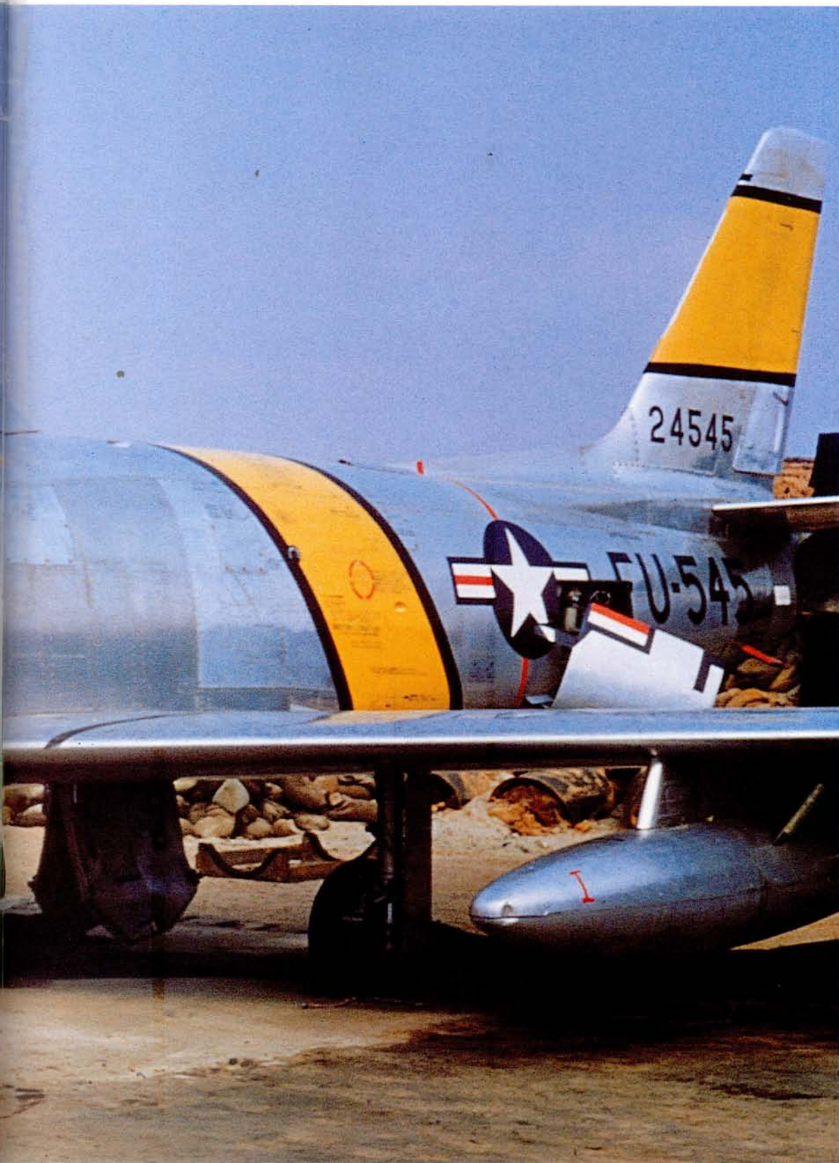
Lt Don 'Dusty' Showen's SCREAMIN' EAGLE is seen ready for the next day's mission in its revetment at Kimpo. The 334th FIS was re-equipped with F-86Fs in early spring 1953. These aircraft could reach the MiG's high cruising altitude, enabling the USAF to score kills that would have been impossible with the earlier A- and E-models (Don Showen)
